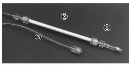
The PicoNozzle holds a microinjection pipette during microinjection. It features good stability, minimum dead volume for fast response, and allows pipettes to be changed quickly and easily.
